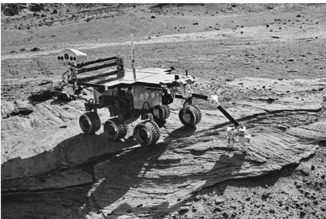
**Fig. 2** The Field Integrated Design & Operations (FIDO) rover performs manipulator operations during a field trial designed to closely emulate Mars mission operation scenarios in Martian-like terrain
